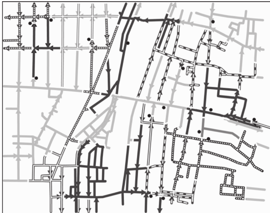
Figure 23.9 The inward directed Voronoi diagram generated from parking lots in Kyoto, Japan.
