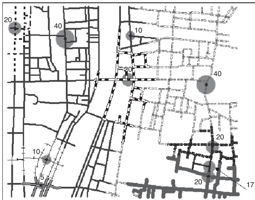
Figure 23.10 The additively weighted network Voronoi diagram generated from convenience stores in Kyoto, Japan (each circle indicates its weight \eta_i ).
