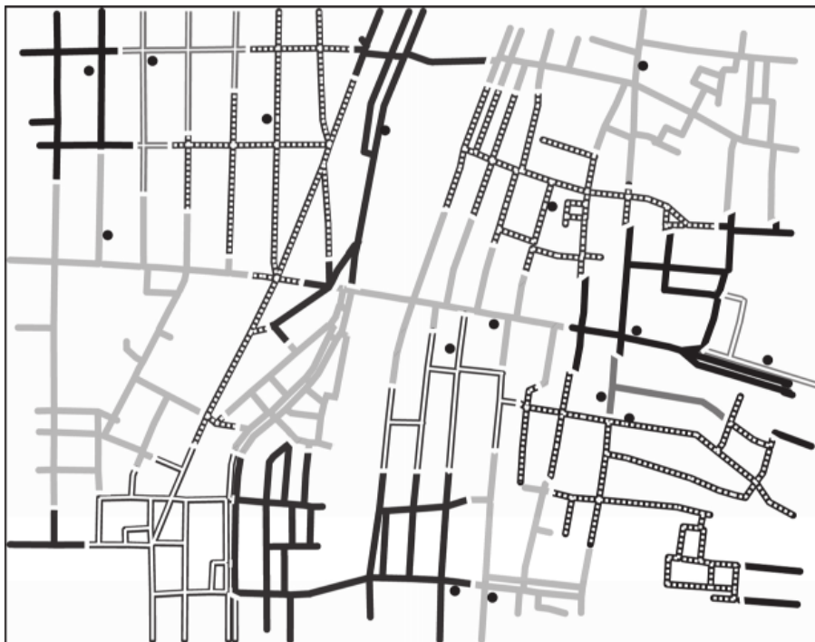
Figure 23.7 The ordinary network Voronoi diagram generated from parking lots in Kyoto, Japan.
