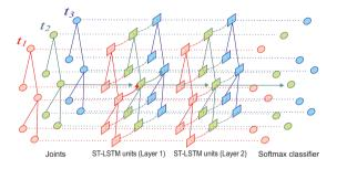
**Fig. 3.** A graphical model of the deep tree-structured ST-LSTM network. For clarity, some arrows are omitted in the stacked network (better viewed in color). In this figure, the output of the first ST-LSTM layer is fed to the second ST-LSTM layer as its input. The second ST-LSTM layer's output is fed to softmax layer.
