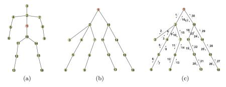
**Fig. 2.** (a) Skeletal joints of a human body. In the simple joint chain model, the joint visiting order is 1-2-3-...-16. (b) Skeleton is transformed to a tree structure. (c) Tree traversal over the spatial steps. The tree can be unfolded to a chain with the traversal, and the joint visiting order is 1-2-3-2-4-5-6-5-4-2-7-8-9-8-7-2-1-10-11-12-13-12-11-10-14-15-16-15-14-10-1.
